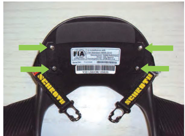
Figure 2 – Screws fixing the tether carriers part can be accepted
