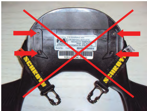
Figure 1 – Without screws fixing the tether carriers part must not be accepted
